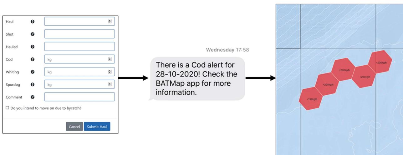
**Figure 2:** Schematic representation of the alerting system. The catch data is entered for each haul in the “Haul” tab. If the catch exceeds the ATV then it automatically triggers a SMS message to be sent. An SMS message prompts the user to open the BATmap app where the most recent alert is automatically displayed.
