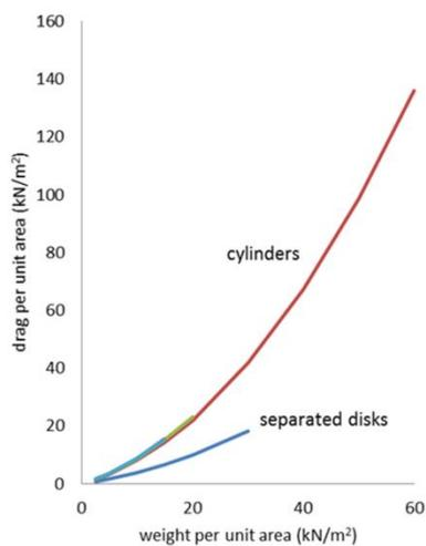
**Figure 12.** The regression lines to the cylindrical element data on the soft sediment are almost indistinguishable for each of the  $d/b$  categories. However, there is a difference between the cylinders and the separated disks.
