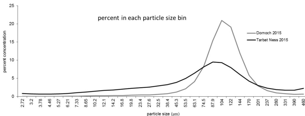
**Figure 10.** The percent concentration of sediment in each of the 32 logarithmically increasing particle size bins at the two sites where the sledge was towed.
