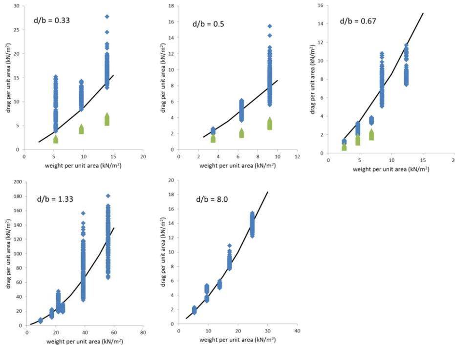
**Figure 11.** The geotechnical drag measurements where the blue diamonds are the data from the softer sediment east north east of Tarbat Ness and the green triangles are from the sandier sediment in the Dornach Firth. The black lines are the regression curves to the data collected in the softer sediment site estimated at a towing speed of  $U = 1.54 \text{ ms}^{-1}$ .
